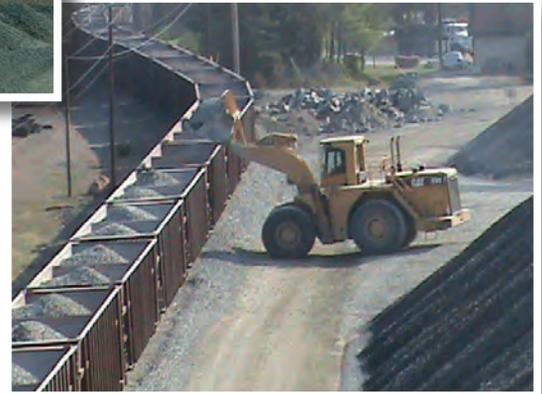
*Sunrock's flood-loading system allows for 60 Herzog rail cars (100 tons each) to be loaded and moved out by Norfolk Southern in 2.5 to 3 hours.*
