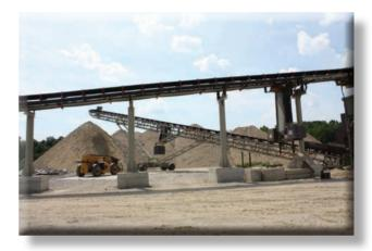
projects specific objectives as well as overcome the site issues, the team determined the primary plant needed to be substantially upgraded and relocated. In addition, a significant amount of conveyors had to be constructed and installed, and the back half of the production plant had to be entirely reconfigured and enhanced.
